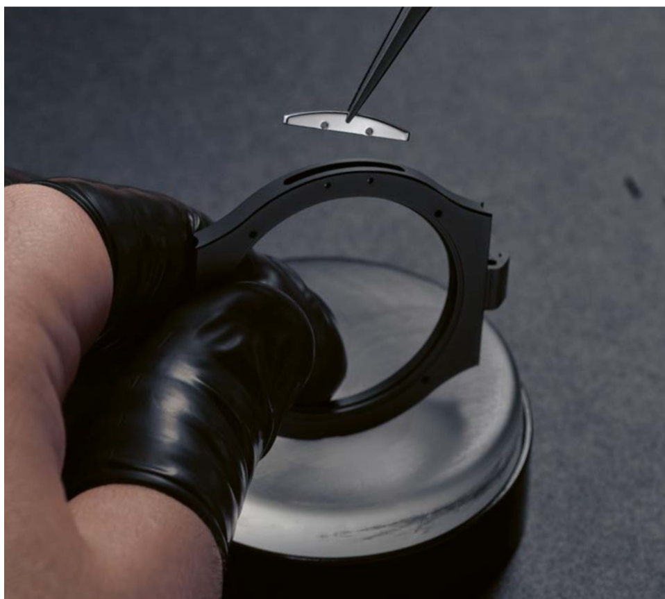
Assembly of the tantalum inserts on the case middle of the Chronomètre Furtif.
