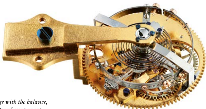
2. Detail of Breguet's natural escapement.
