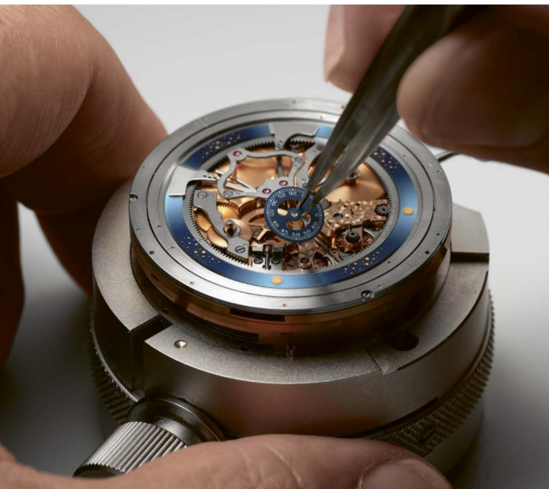
Positioning and adjustment of the seconds disc during the assembly of the Astronomic Souveraine movement.
