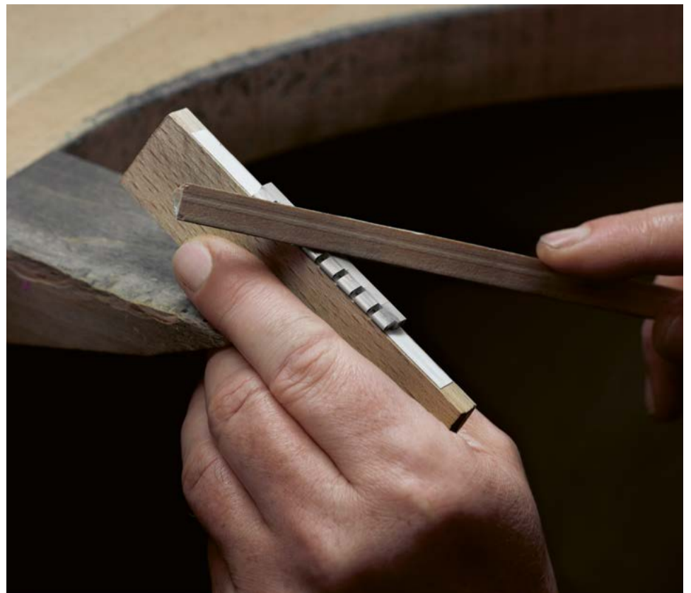
Preparation of bracelet finishes. Each component of the case receives the same level of attention. Before reaching the final finishing operations, the links of the platinum lineSport bracelet are patiently prepared by hand.
