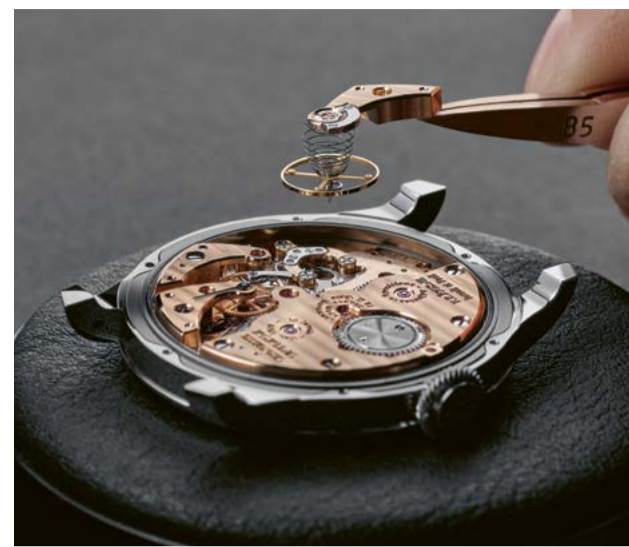
Assembly of the balance and its bridge on the Chronomètre Optimum movement. The watchmaker can then adjust the regulating organ, the balance point of the movement, in interaction with the EBHP escapement.
