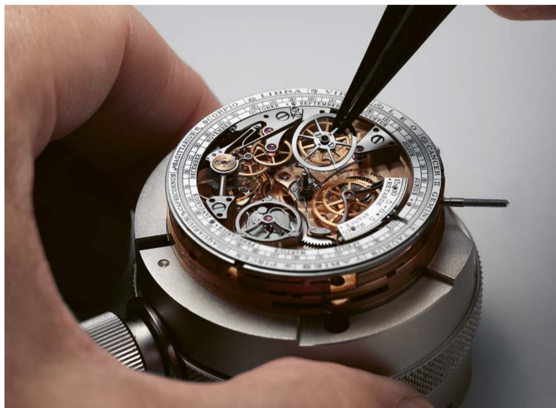
Fitting of the equation of time cam on the back of the Astronomic Souveraine movement.
